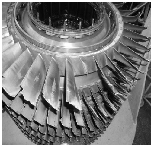
Fig. 3. External appearance of the gas-turbine drive compressor after entry of associated gas liquid fraction into the combustion chamber.
