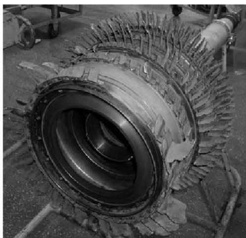
Fig. 3. External appearance of the gas-turbine drive compressor after entry of associated gas liquid fraction into the combustion chamber.
